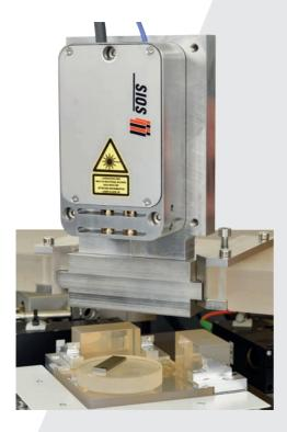
the resolution or stability of the measurement. The length resolution of the interferometer is 5 pm and this can be achieved even under normal laboratory conditions thanks to the differential principle of the measurement system.
